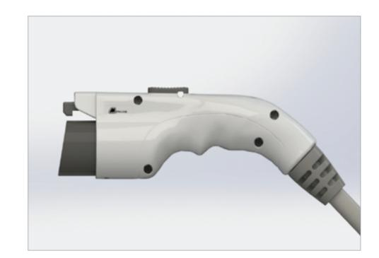
The ergonomic contoured grip and strain relief makes the connector comfortable and easy to use. The Methode custom cable remains flexible, even at low temperatures The cable construction for the 40A and 32A coupler is 3x 10AWG, 1x 18AWG. For the 20A and 16A coupler it is 3x 14AWG, 1x 18AWG. Also available with other types of cable.
