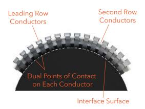
Each copper alloy beam includes a slight indentation in the finger tip to create dual contact points, adding to the massively parallel contact points.
